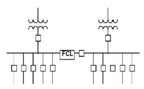
Figure 5: Fault current limiter in the bus tie position. The two buses are tied, yet a faulted bus receives the full fault current of only one transformer.
