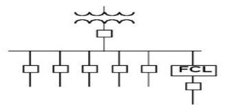
**Figure 4:** Fault current limiter in the feeder position. The fault current limiter FCL protects an individual circuit on the bus. Underrated equipment can be selectively protected as needed in this manner.
